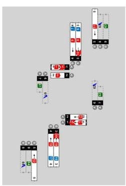
The above linking works when the junction has no queues on the internal reservoirs, with no delay between a controlling stage ending ROW and the new controlling stage (on the opposite stream) gaining ROW. This reduces the cycle time when the queueing on the circulatory is not causing an issue.
